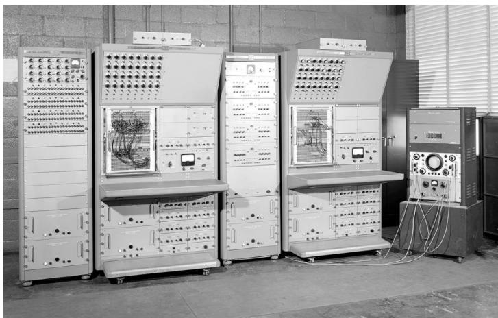
PACE 16-31R, 1950s Electronic analog computer, Electronic Associates Inc., NASA's Lewis Flight Propulsion Laboratory, Used in Mercury, Gemini, and Apollo programs.
