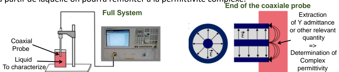
Figure 1 : Liquids characterization system and end of the coaxial probe with electromagnetic fields illustration
